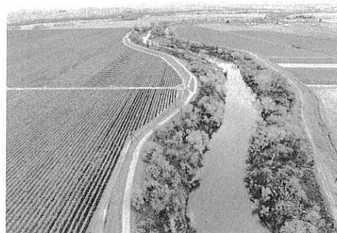
A drone photo shows a recharge project in Sacramento County. Diverted water is infiltrated to groundwater storage in the underlying, critically overdrafted South American and Cosumnes Groundwater Subbasins. Photo taken February 8, 2024. Sara Nevis / California Department of Water Resources
